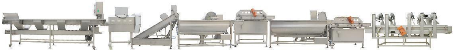
Leafy vegetable cutting and washing production line
